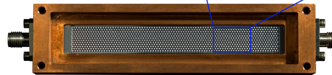
Microlens arrays for FIRESS, developed at GSFC
