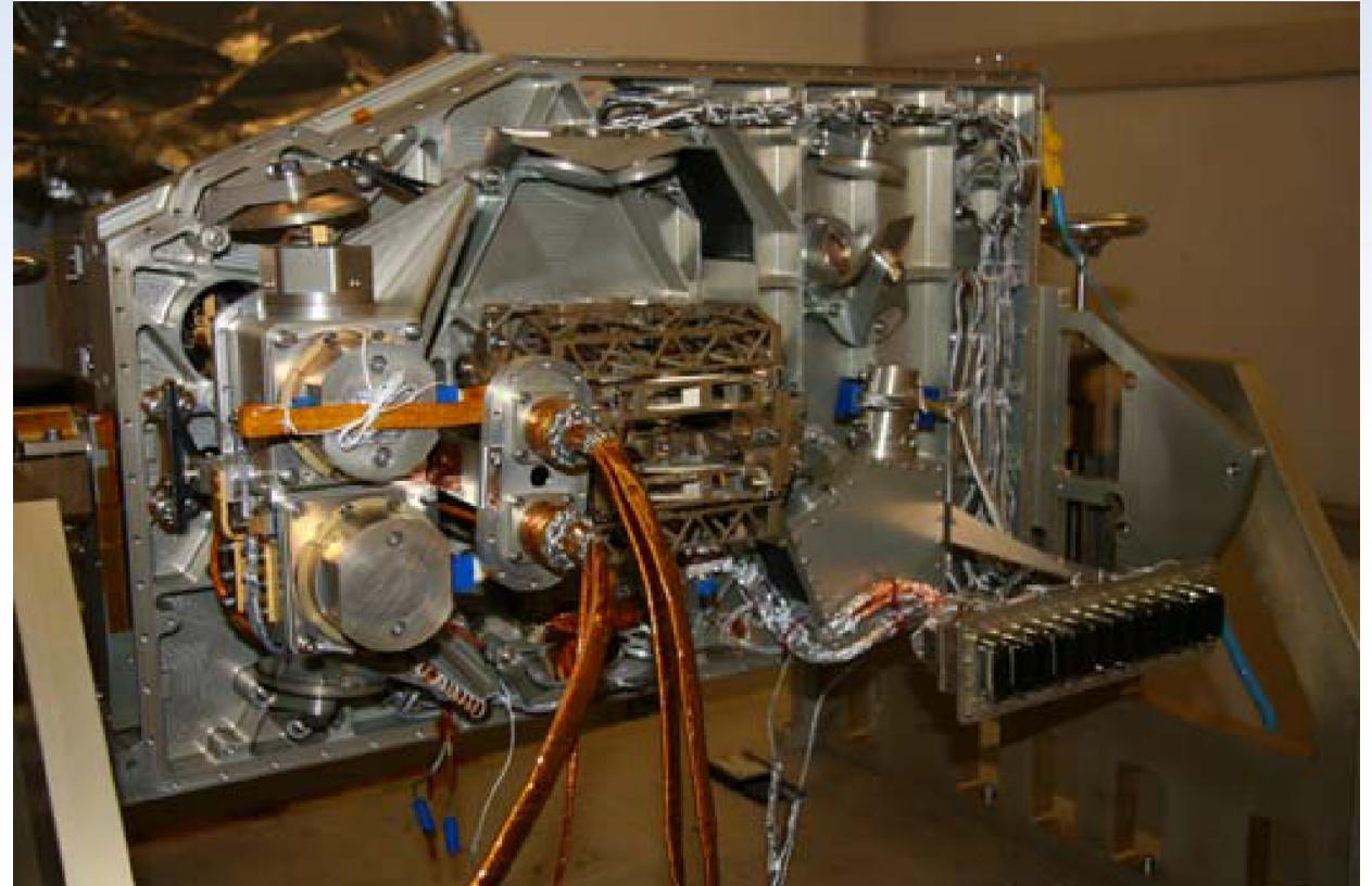
Herschel SPIRE FTS. PRIMA FIRESS FTS team uses the same team for the scan mechanism. FIRESS much more sensitive with cold telescope and narrow band on detector.
