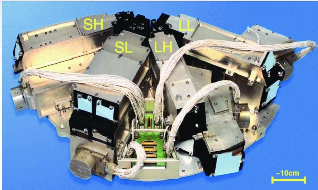
Spitzer Infrared spectrograph -> all aluminum grating modules with no moving parts. Houck et al.
