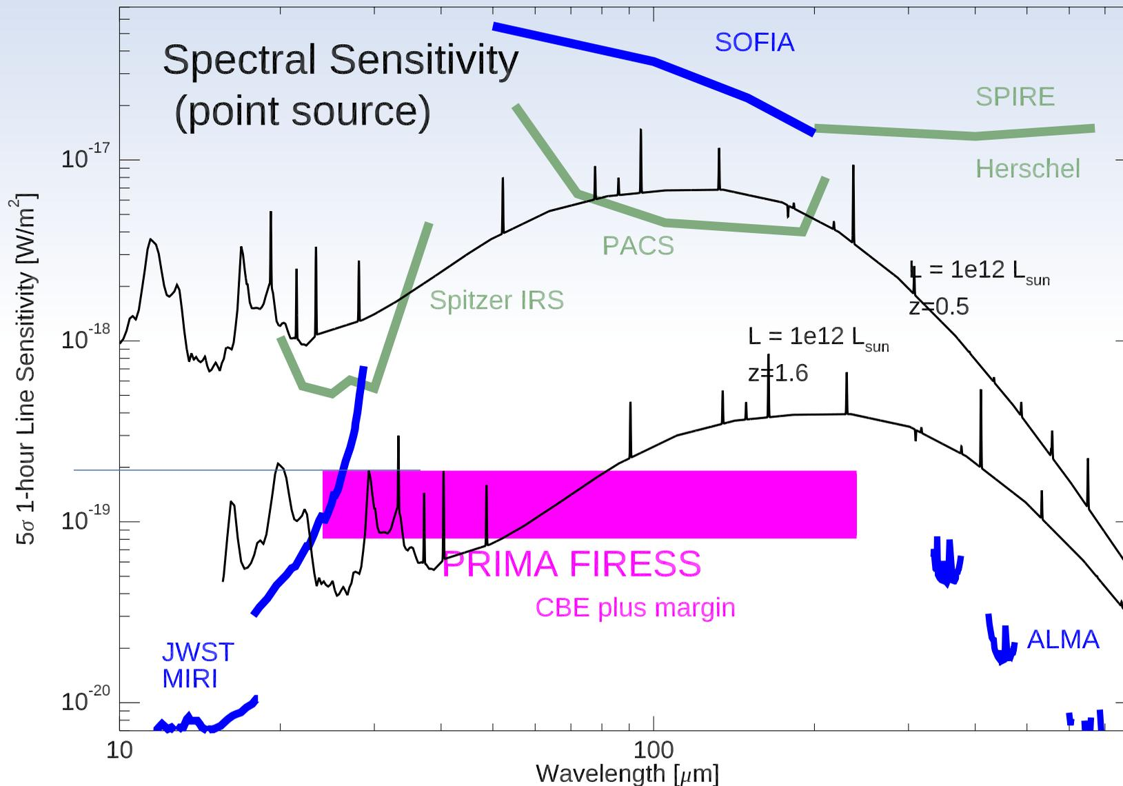
Low-res base grating mode provides  $R \sim 130$  and covers band shown. **24 to 239 microns**
